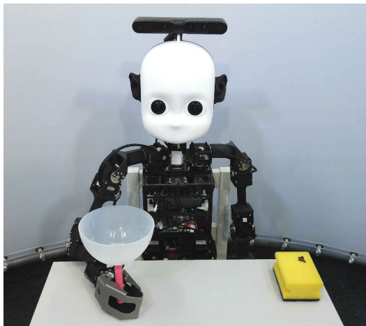
Fig. 2. Cleaning scenario with the NICO robot. Our scheme is composed of two objects, 3 locations, and 7 action classes.
